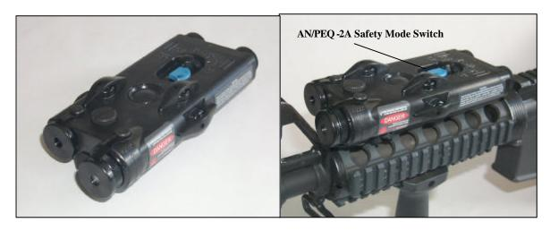
The Infrared Target Pointer/Illuminator/Aiming Laser, (ITPIAL) incorporates lessons learned with Aiming Lights in Desert Storm, other combat operations, and extensive field evaluation, plus production experience with over 50,000 US Military standard aiming lights. The result is a dual beam multi-function laser, which combines the utility and operational effectiveness of aiming lights and illuminator/pointers in a singe device.
