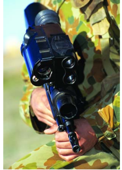
AICW fitted with the sophisticated Vingsight that provides a range of 'Forward Observer' type systems to the soldier and their weapon. (DSTO)
