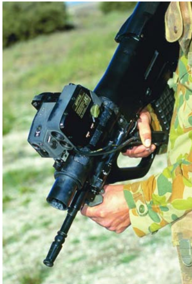
This AICW is fitted with the ITL Viper Multi-Purpose Rifle System, ITL provided significant in-kind support to the demonstrator with their multi-function laser capability. (DSTO)
