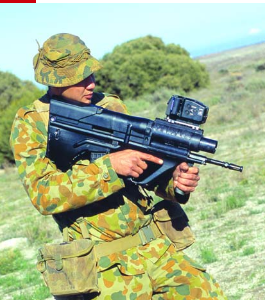
Above: Vision of the future? An Advanced Individual Combat Weapon combining magazine feed 5.56mm and 40mm is demonstrated in the hands of an Australian soldier. (DSTO)
