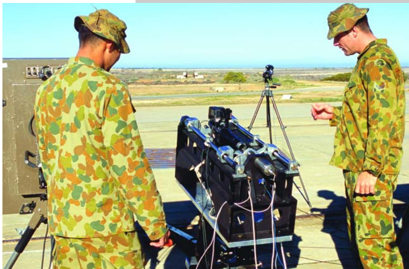
The AICW demonstrator is readied for firing at the Proof and Experimental Establishment, Port Wakefield, from a trainable testbed. Performance was high despite being a concept demonstrator. (DSTO)
