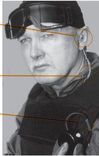
Invisio bone whisper mic and speaker are totally contained within a custom or universal earmold. Optional hearing protection or peripheral hearing filter.
