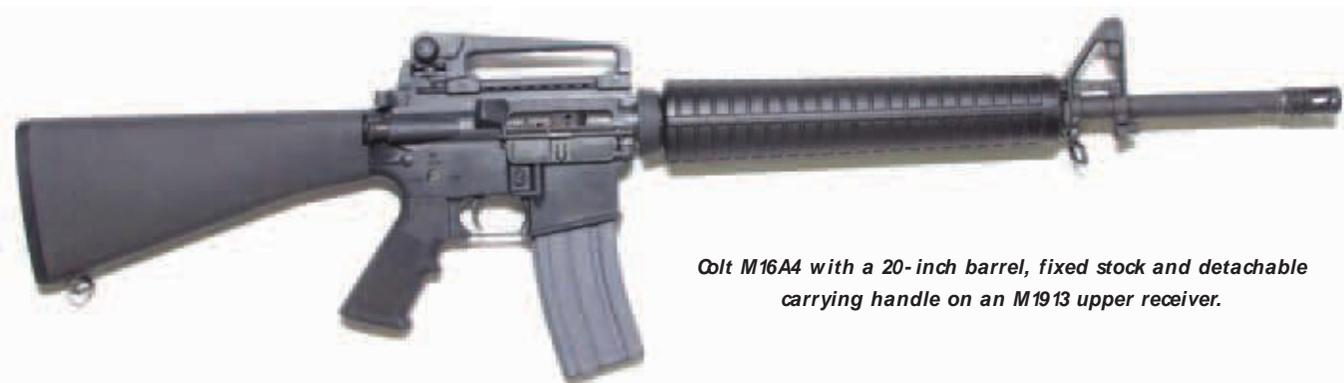
*Colt M16A4 with a 20-inch barrel, fixed stock and detachable carrying handle on an M1913 upper receiver.*
