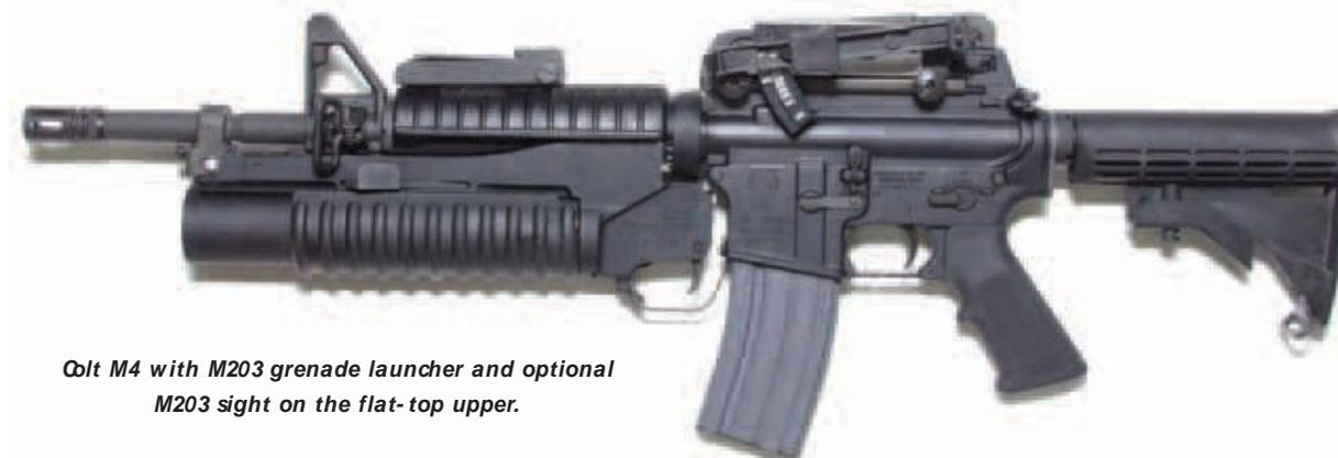
*Colt M4 with M203 grenade launcher and optional M203 sight on the flat-top upper.*
