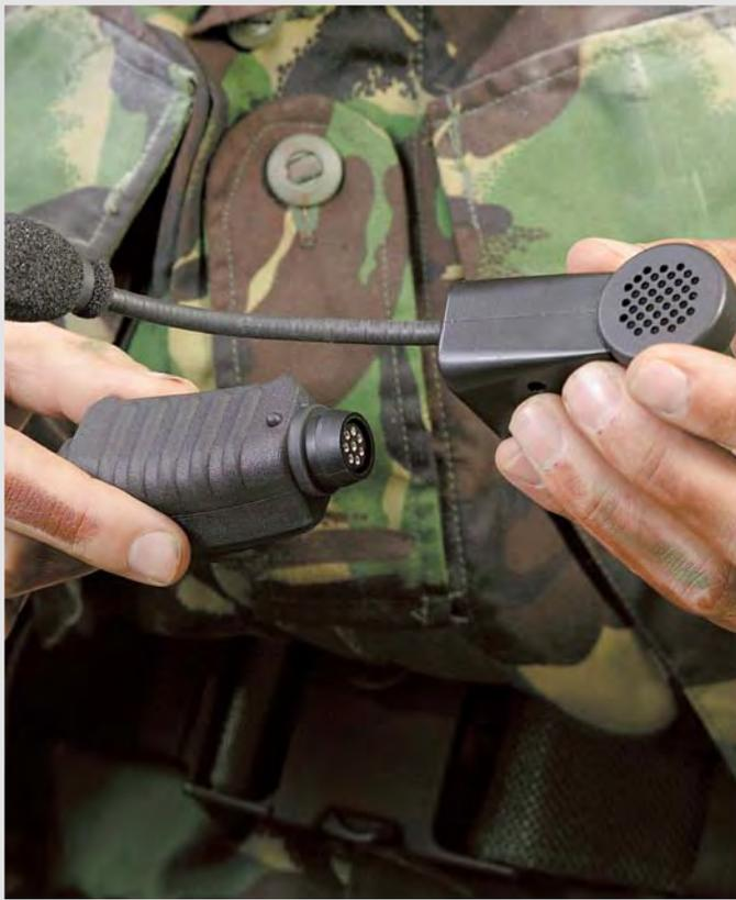
*The Skeletal Handset is easily assembled by snapping together the handset assembly and the standard pressel. When not being used, the Skeletal Handset can be folded up and kept in a jacket pocket or webbing pouch.*
